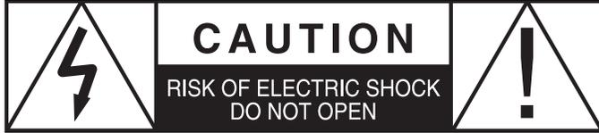
**CAUTION:** To reduce the risk of electric shock, do not remove the cover (or back). No user serviceable parts inside. Refer to qualified personnel.
