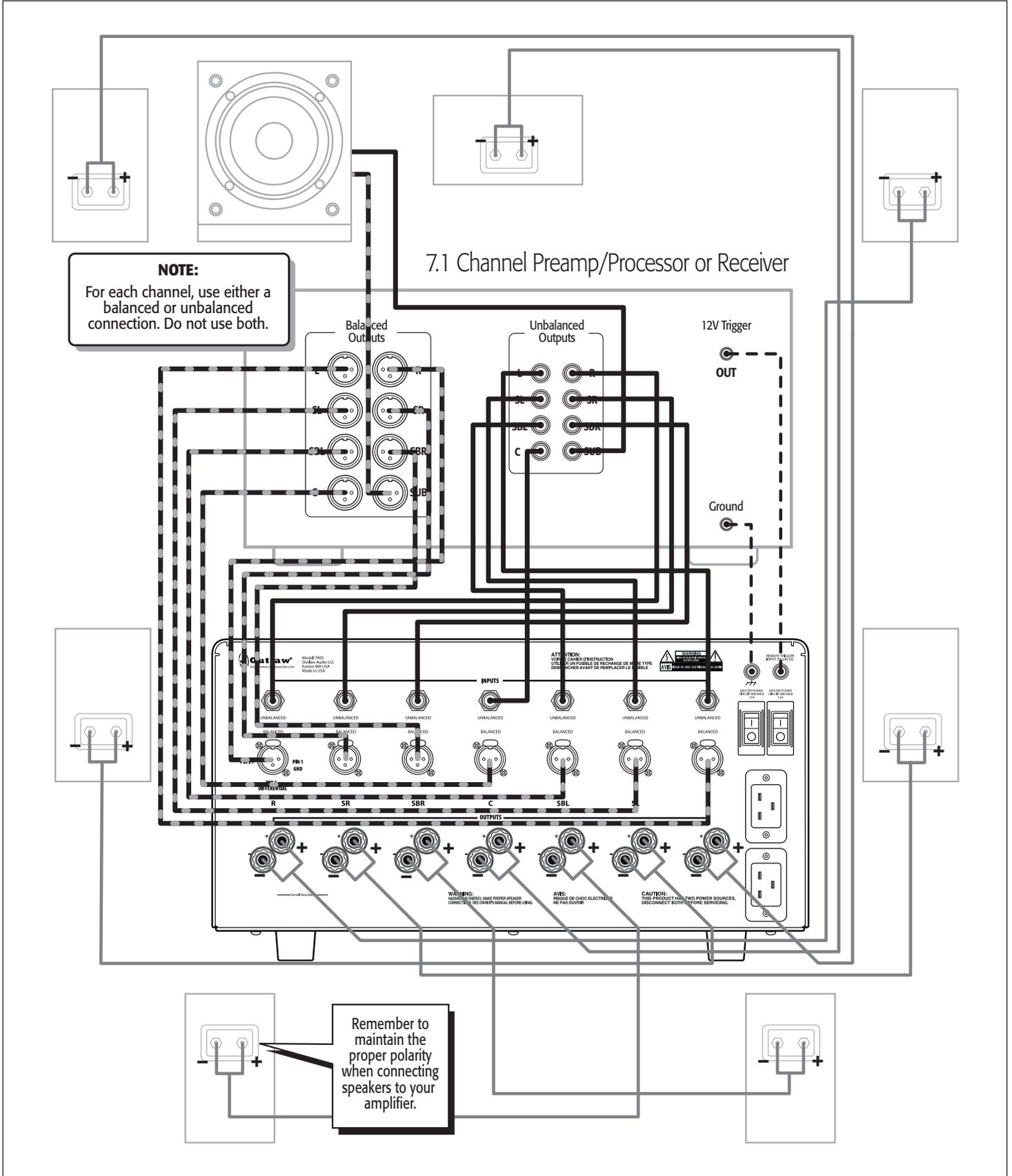
When using banana plugs, connections may be made by simply inserting the jack affixed to your speaker wire into the hole provided on the rear of the colored screw caps on the binding posts. Before using banana type jacks make certain that the plastic screw caps are firmly tightened down by turning them in a clockwise direction until they are snug against the chassis. This will insure that the maximum surface area of the plug is in contact with the jack. Be certain to observe proper polarity.
