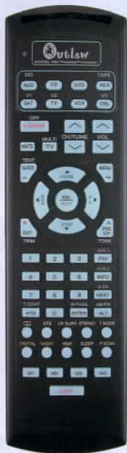
▲ The supplied universal learning remote is backlit and features a large volume control.
