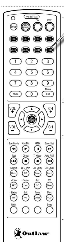
PLEASE NOTE: To operate the functions of the Model 975, access the setup menus, or select a source input, you must first press the TNR button. Once pressed, you can directly control the functions of the Model 975 indicated by the labels printed above each button on the remote.
