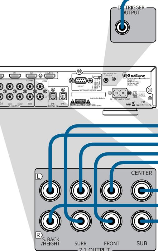
**➤ IMPORTANT NOTE:** Before attempting to plug any jacks into any power amplifier verify that the power amplifier is turned off and/or disconnected from the AC power. Failure to do so can potentially result in severe damage to your amplifier and loudspeakers.
