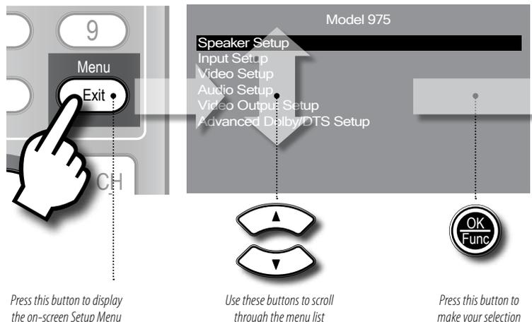
Press this button to display the on-screen Setup Menu
