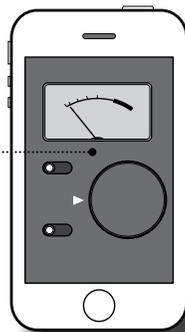
The Level Calibration menu is shown above. Use this menu to set the individual output level of each speaker in your system. Adjusting these settings can compensate for room effects, as well as for speakers placed different distances from the listening area, ensuring a more natural and accurate soundfield.
