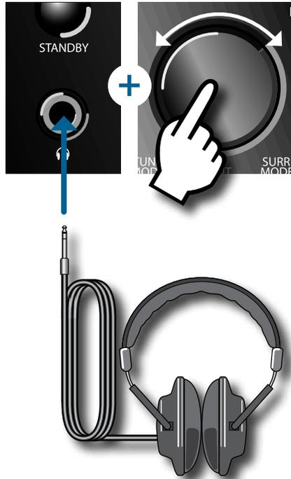
The Model 975's front headphone jack works with any standard headphones equipped with a 1/4-inch plug, or headphones equipped with a 1/8-inch plug and used with a 1/8- to 1/4-inch adapter.
