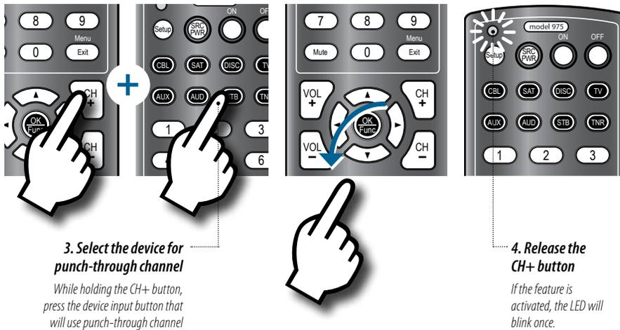
3. Select the device for punch-through channel
