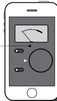
The Model 975 allows you to adjust channel levels two ways: while listening to source material during playback, or by using the internal test tone. Either method makes it easy to adjust the channel levels.
