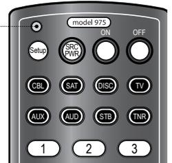
The Macro Power mode enables the remote control's power button to turn on two devices: first the selected device, then a second device about 1 second later. For Macro Power to work, the remote must already be programmed to control both devices.
