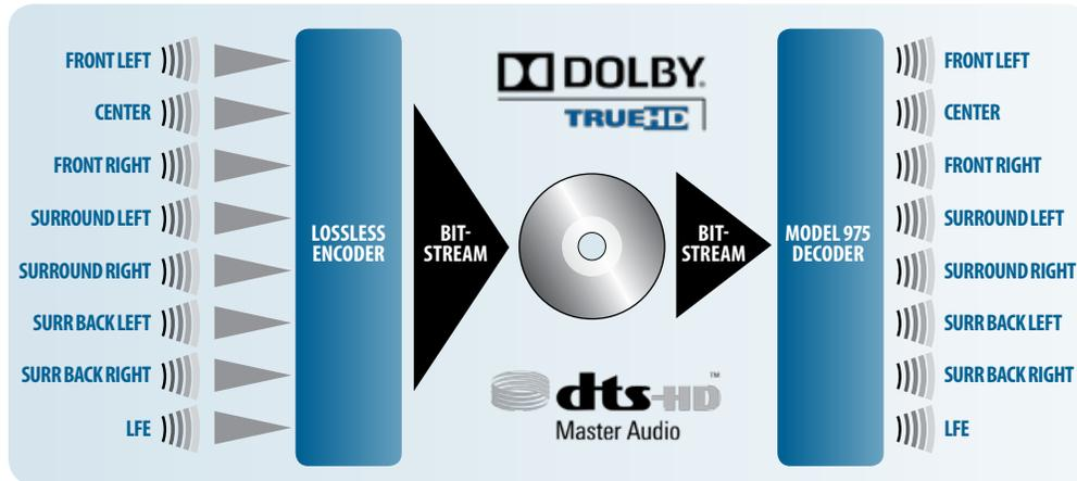
bitrates. This format can only be delivered to the receiver in its native form via HDMI or transcoded to Dolby Digital 640 kbps for output via coaxial or optical digital audio.
